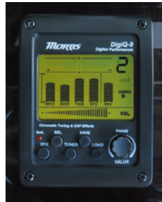
Morris DigiQ-9 Preamp : Volume, 3-band EQ, Phase, Delay, Chorus, Flanger, Tremolo, Reverb, Tuner
